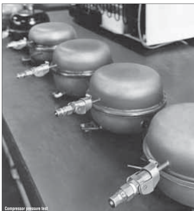
Compressor pressure test
